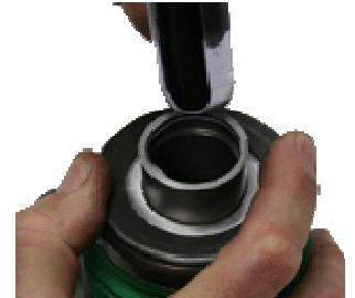
11. Install spring. 12,13,14. Install RPS piston and push down on spring. Re-install retaining clip and tap
