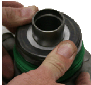
11. Install spring. 12,13,14. Install RPS piston and push down on spring. Re-install retaining clip and tap
