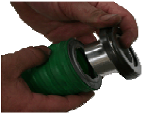
5 & 6. RPS piston does not fit without grinding the small metal tabs away. 7. Finished
