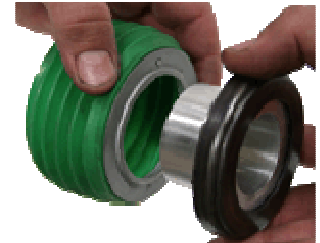
5 & 6. RPS piston does not fit without grinding the small metal tabs away. 7. Finished
