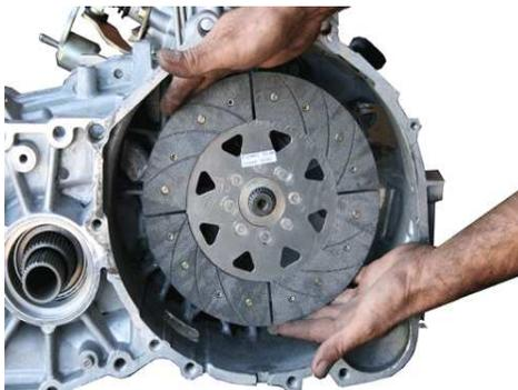
Please slide the disc(s) on the input shaft and make sure they move freely. Do not be afraid to coat the splines with a little more anti-seize to prevent hard spots, but be sure to wipe off the excess. Make sure the splines are free of any burrs or imperfections.
