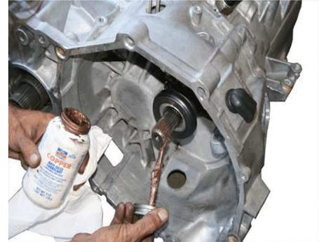
Please clean the input shaft thoroughly prior to installing your new RPS Clutch. To insure an easy installation, apply a thin layer of Anti-Seize on the input shaft as well as the inside of the clutch hub(s). We prefer copper Anti-Seize over silver for long term use. Please use sparingly as excess will contaminate friction surfaces and cause unnecessary slippage.
