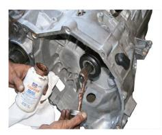
Torque ARP Flywheel bolts to 80FT/LBS and use a dab of Red Loctite on each bolt. When factory bolts are used please refer to factory specs.
