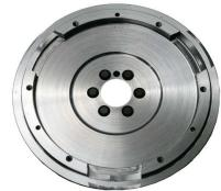
Common Torque Specs: ARP Flywheel bolts: 80 ft/lbs Clutch cover bolts: 25-28 ft/lbs Factory Flywheel bolts: Use factory torque specs.
