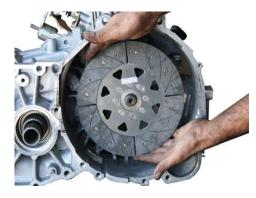
Please slide the disc(s) on the input shaft and make sure they move freely. Do not be afraid to coat the splines with a little more anti-seize to prevent hard spots, but be sure to wipe off the excess. Make sure the splines are free of any burrs or imperfections.
