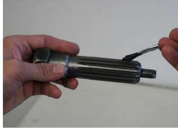
***Clean and remove all dirt and rust from the input shaft and then apply a small layer of lapping compound.***
