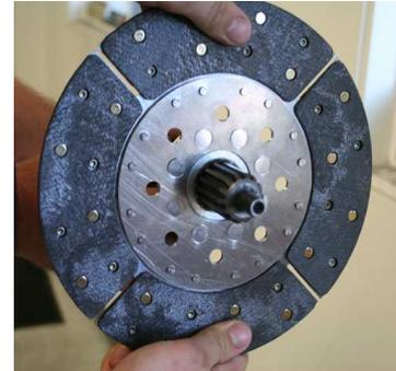
***Slide each disc, one at a time, back and forth on the input shaft. This action removes any burrs or imperfections from both the clutch hub and input shaft.***
