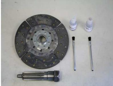
***RPS supplied lapping compound and grease with brushes. (Input shaft in picture is for illustration only).***
