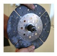
Slide each disc, one at a time, back and forth on the input shaft. This action removes any burrs or imperfections from both the clutch hub and input shaft.
