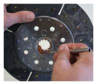
Make sure to completely clean and remove ALL lapping compound from each disc hub and the input shaft with a wire brush. Using a new brush, apply an even layer of grease onto the input shaft and inside each clutch hub. Slide each disc back and forth onto the input shaft and wipe off any excess grease that could fling up onto the clutch facings. ENJOY a smooth working clutch!
