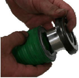
5 & 6. RPS piston does not fit without grinding the small metal tabs away. 7. Finished
