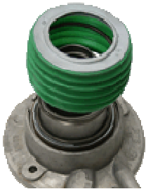
11. Install spring. 12,13,14. Install RPS piston and push down on spring. Re-install retaining clip and tap
