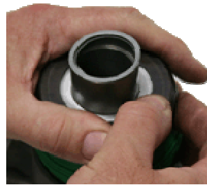
11. Install spring. 12,13,14. Install RPS piston and push down on spring. Re-install retaining clip and tap
