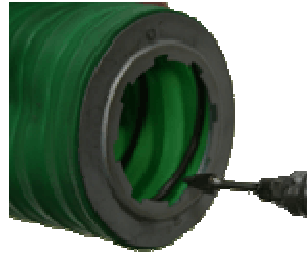
5 & 6. RPS piston does not fit without grinding the small metal tabs away. 7. Finished
