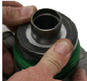
11. Install spring. 12,13,14. Install RPS piston and push down on spring. Re-install retaining clip and tap
