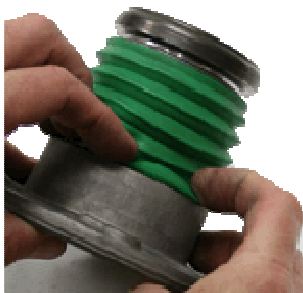
15 & 16. With your fingers push the end of the green boot back inside the stock TOB.
